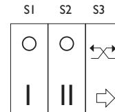
S3 switch activates the "Free cooling" (Bypass) mode , which stops alternate flow and keeps the fan in "extract-only" or "intake-only" mode, to avoid the heat exchange when necessary. To set the "extract-only" mode or "intake-only", place the integral jumpers as per fig. 21A or Fig. 21B. The front cover LED indicates when the Free cooling mode is on.
